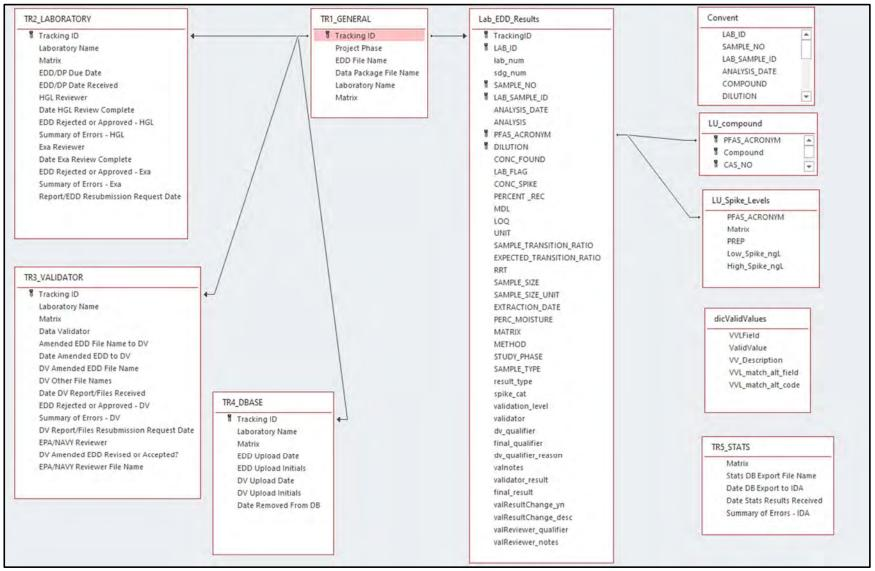
Figure 4. Entity-Relationship Diagram (ERD) for the Project Database
