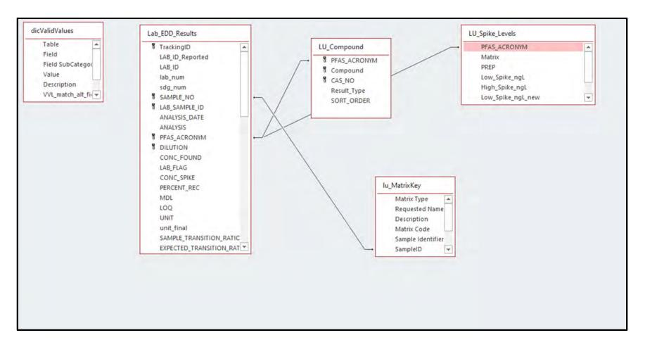
Figure 2. Revised Entity-Relationship Diagram (ERD) for the Project Database
